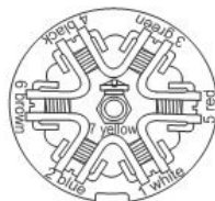
7-way trailer plug - car end-rear view
